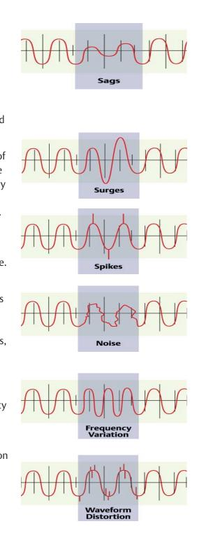
Figure 2. System protection must be ready to handle a wide array of power fluctuations. The illustrations show waveforms for typical 60 Hz AC power. The left and right unshaded areas show how the waveform should look; the shaded area shows how the disturbance distorts the waveform.
